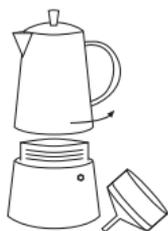
1. Unscrew the coffee maker by holding the lower part and turn the upper part counterclockwise. Remove the funnel.
