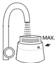
2. Fill the lower part of the coffee maker with water to a maximum below the safety valve. **Attention!** The safety valve must not be under water.
