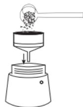
3. Reinsert the filter. Fill it with not too finely ground espresso powder. Do not press the powder firmly down, just smooth it out! Clean the edge of the screw thread of excess espresso powder.
